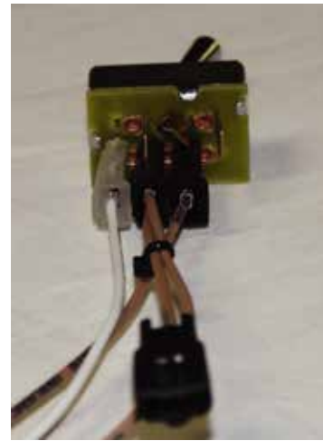
Figure "F" Dual fuel tank switch connection
